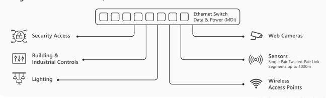
Figure 3: Single Pair Ethernet has the ability to supply power to a wide range of IoT devices
